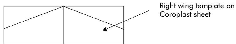
5. With a pair of scissors cut along the diagonal lines. Remove and save the smaller pieces for the vertical stab and canard.
