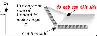
13. Insert the Canard adjustment screw in the hole made in the Canard in step 9, with the hinge cut facing down. Screw the canard with the adjustment screw in the fuselage hole just above the base of the nose. Remove the backing from the glue tape on the fuselage nose. Line up the Canard so the point is in about the center of the nose.
