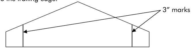
8. Now it is time to bend the winglets. Lay the wing on a table and extend the wing tip past the table edge about 3". Lay a square or a ruler along the same pencil line from the above step. Pushing down on the ruler with one hand and bending the wing tip up with the other. Bend each winglet to 90 degrees. For flight, bend winglet back down to 30 degrees.
