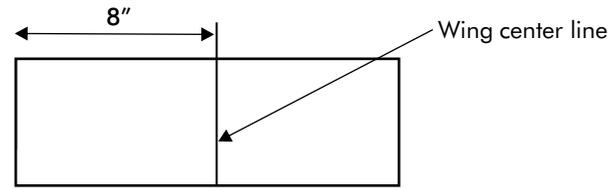
3. Next lay the left wing template over the left side of the Coroplast. Making sure that the template centerline and the Coroplast centerlines are lined up. Use a pencil to mark the left wing.
